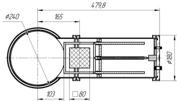
*Tentative design (by BSU Group) of moving mechanics for Si Beam Profile Detectors*
