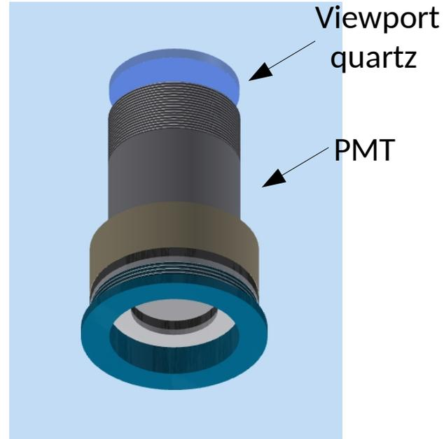
Parts of 3d design of PMT mount
