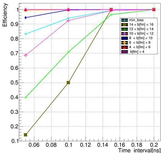
Centrality dependence of T0 efficiency. More than 100 detected photons (QE folded in) in time windows of 50, 100, 150, 200 ns.
