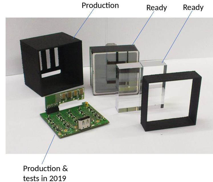
4 quartz bars  $28 \times 28 \times 15 \text{ mm}^3$  in every FFD module
