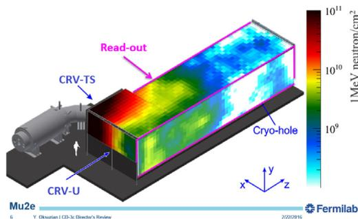
Fig. 1. Expected distribution of neutron fluences [10].
