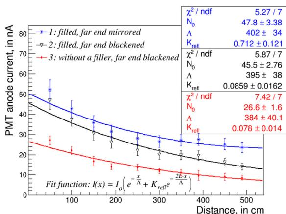
Fig. 9. Light yield as a function of the distance from the PMT for the 5 m long strip irradiated by the radioactive  $^{60}\text{Co}$  source.
