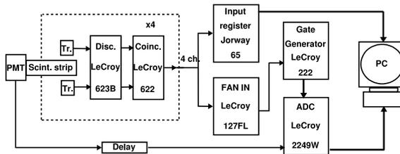
Fig. 7. Block diagram of the electronics used for measurements with cosmic muons.
