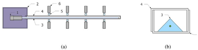
Fig. 6. Layout of the experimental setup (a) and the cross-section of the lightproof Al U-channels with a strip inside (b); (1) EMI 9814B PMT, (2) black box, (3) strip, (4) lightproof Al U-channel, (5) four pairs of  $(20 \times 25 \times 30)$  mm<sup>3</sup> trigger scintillation counters, (6) FEU 85 PMT.
