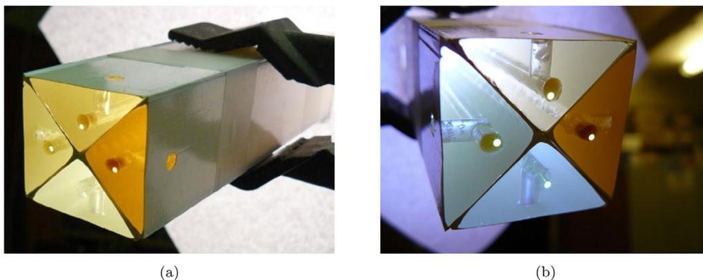
Fig. 13. Unexposed strip is located in the lowest position, followed clockwise by three other strips irradiated by the neutron beam with the fluences of  $1.2 \times 10^{14}$ ,  $3.8 \times 10^{14}$ , and  $16 \times 10^{14}$  neutrons per  $\text{cm}^2$  respectively. The left photo was taken under the illumination by a regular incandescent lamp and the right photo was taken under blue light.
