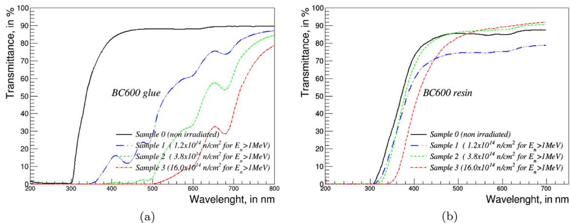
Fig. 12. Transmittance of the BC-600 glue (a) and the BC-600 resin (b) before and after the irradiation by the neutron beam with different fluences.
