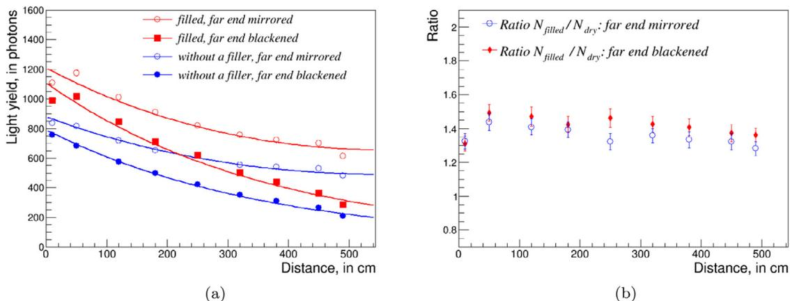
Fig. 3. Simulation results for the light yield from the 5 m long strip with a triangular cross-section (a). Relative increase in the light yield (b).
