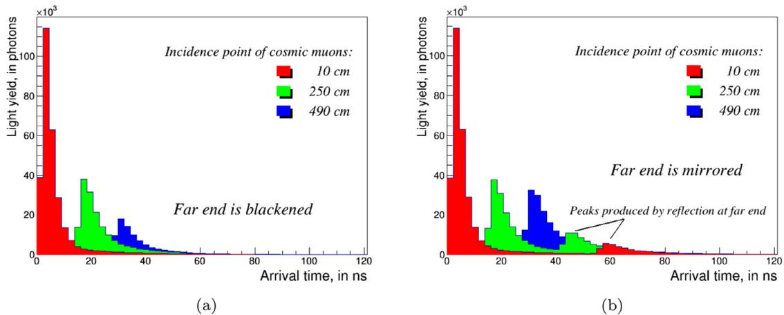
Fig. 4. Simulation results for the light signal arrival at the photodetector from different distances.
