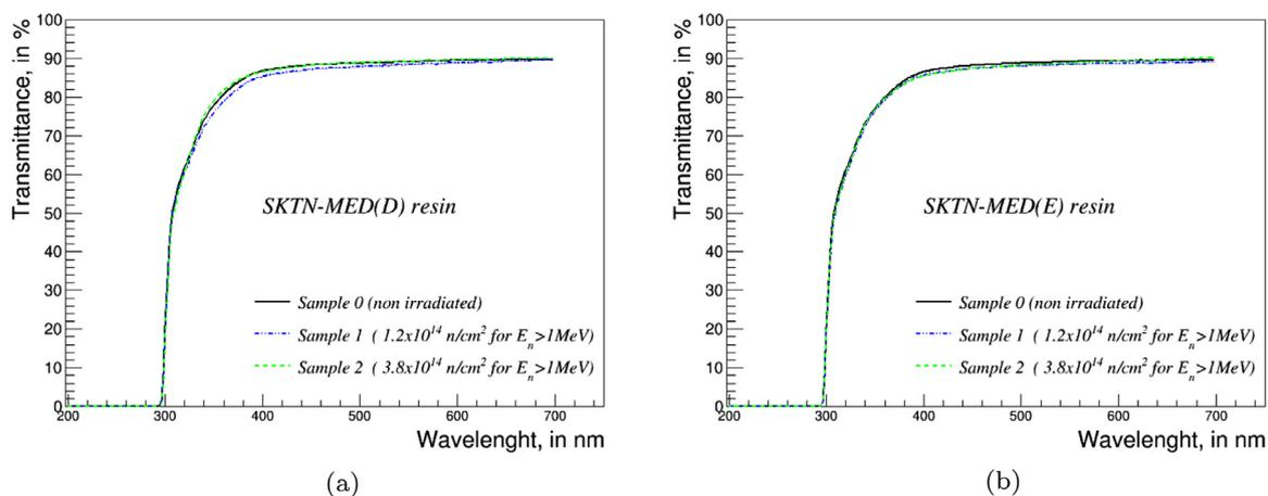
Fig. 10. Transmittance of SKTN-MED(D) and SKTN-MED(E) resins as a function of the light wavelength before and after the irradiation by the neutron beam with different fluences. The Plexiglas window suppressed strong ultraviolet light (less than 300 nm).
