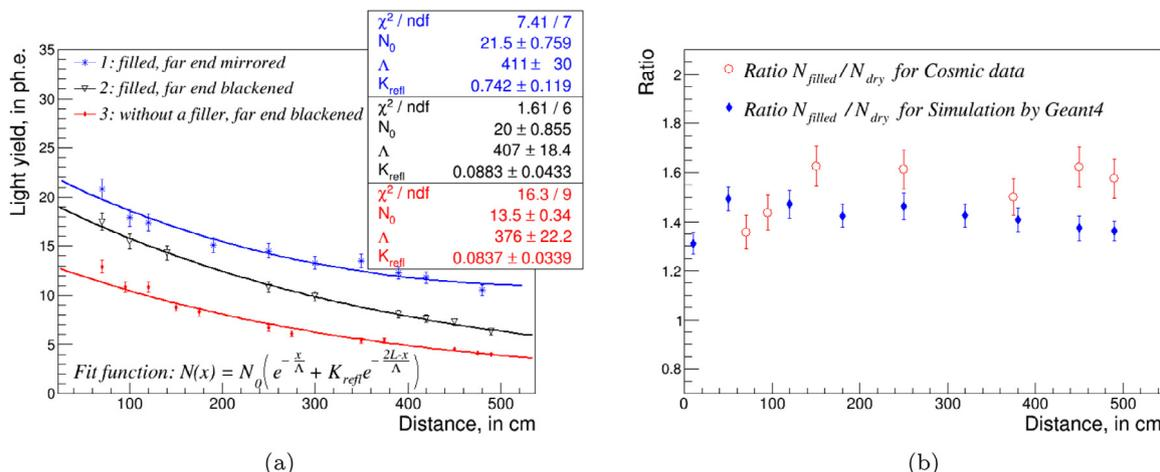
Fig. 8. Light yield (in photoelectrons) of the 5 m long strip on cosmic muons under different conditions of the study (a). The experimental data with the simulation (b).
