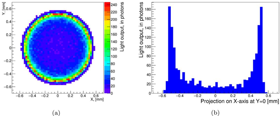
Fig. 5. Light distribution at the WLS fiber end: (a) - 2D distribution chart at the fiber end; (b) - projection on X-axis at Y=0.
