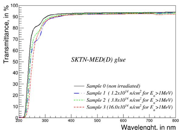
Fig. 11. Transmittance of the sample made of the SKTN-MED(D) glue before and after the irradiation by the neutron beam with different fluences.
