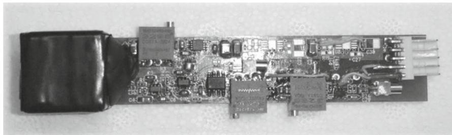
**Fig. 2.** A SensL-SiPM-based trigger counter.
