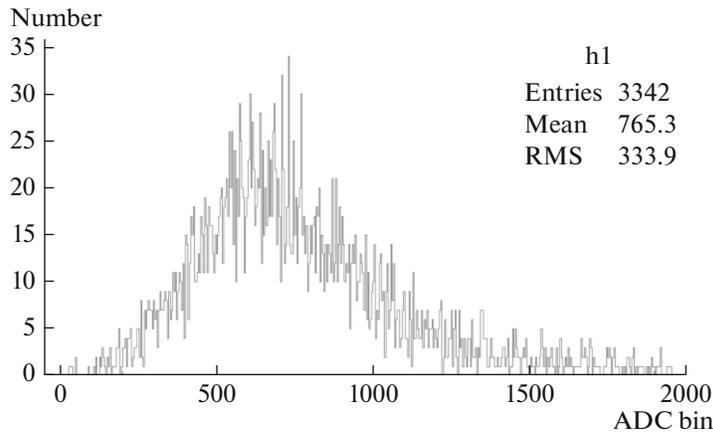
Fig. 4. A typical spectrum of cosmic muons for a triangular scintillation strip.
