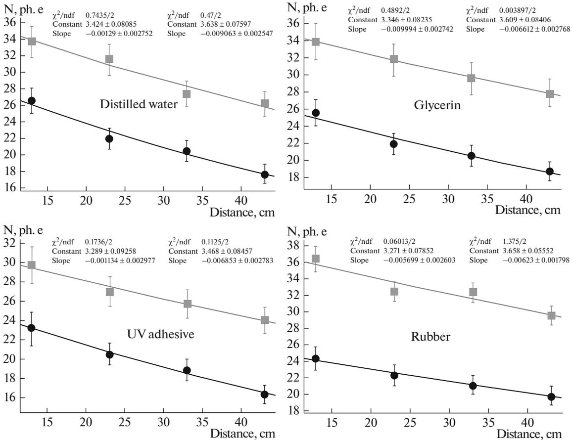
**Fig. 6.** Light collection from strips with fillers of various types. The circles indicate strips without the filler and the squares indicate the strips with the filler.
