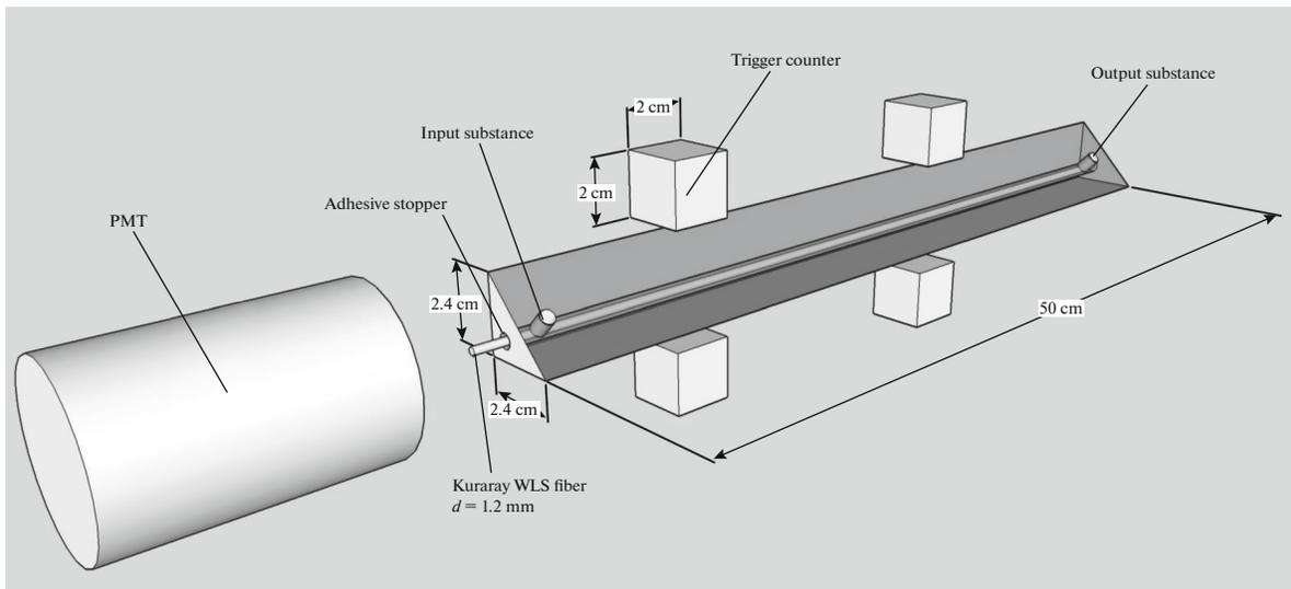
Fig. 3. Schematic arrangement of the components.
