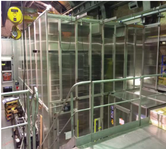
Fig. 1. The Demonstrator of the SuperNEMO under antiradon tent built in the underground laboratory (Modane, France).
