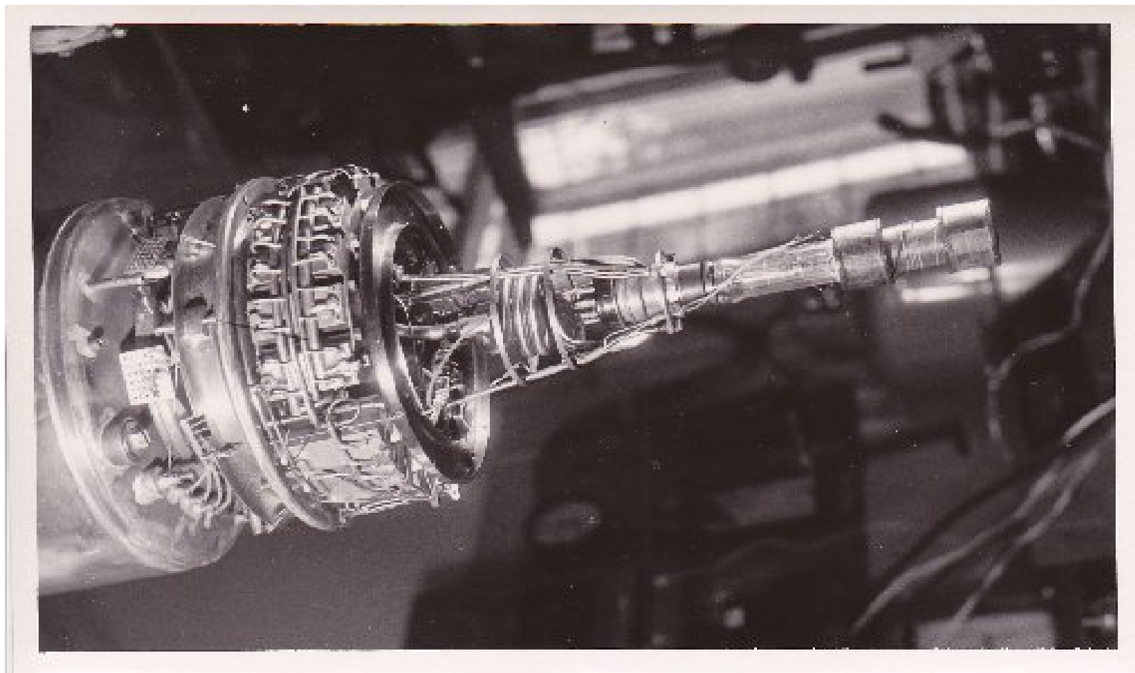
An ultra low part of the cryostat of the dilution refrigerator
