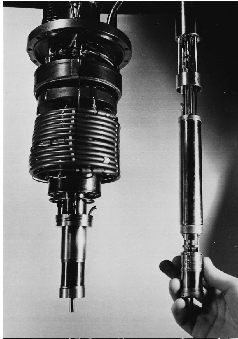
The Low temperature unit of the first Frozen Polarized Target and Insert for loading Target Material.
