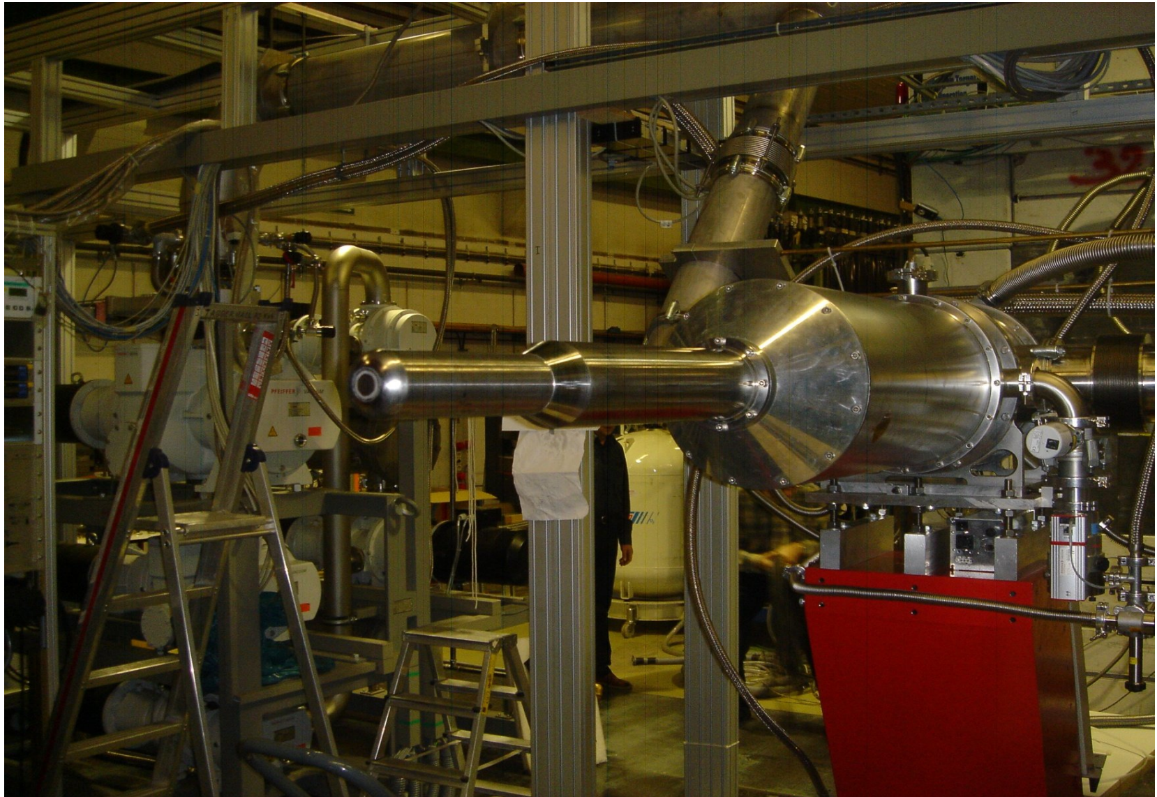
Frozen Polarized Target at MAMI C (Mainz).
