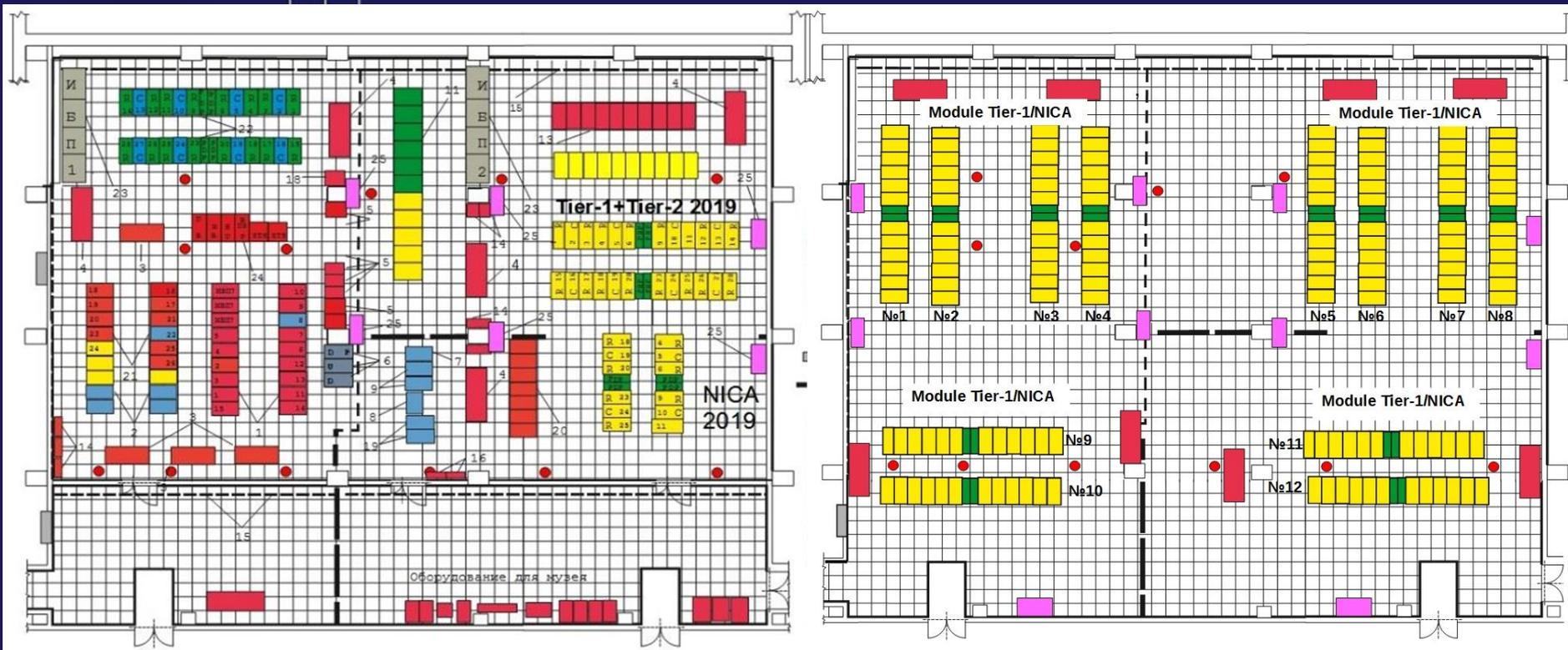
A scheme of arranging the equipment in the computer hall on the 2-nd and 4-th floors
