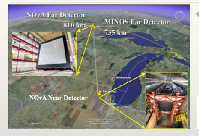
Precision is achieved by placing a detector close to the source (Near Detector) and one at or close to the oscillation maximum (Far Detector)
