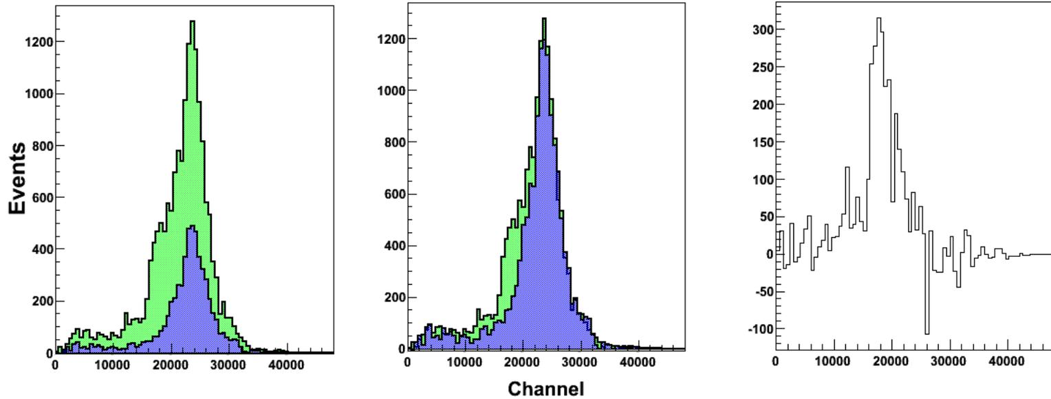
**CH<sub>2</sub>-C subtraction for amplitude spectrum of P-counter.**
