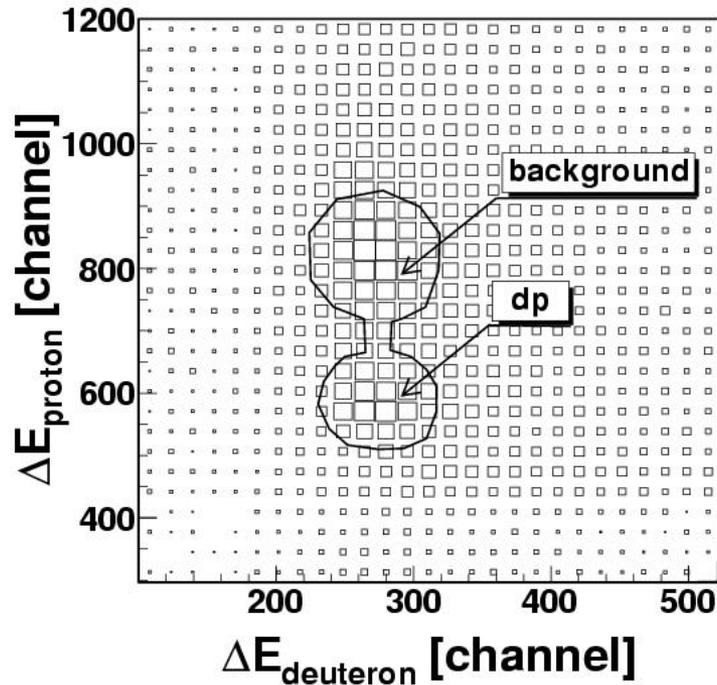
The correlation of the energy-loss signal for a pair of the deuteron and proton detector at 70° in c.m.s. The solid line is a graphical cut for the dp-elastic events candidate selection.
