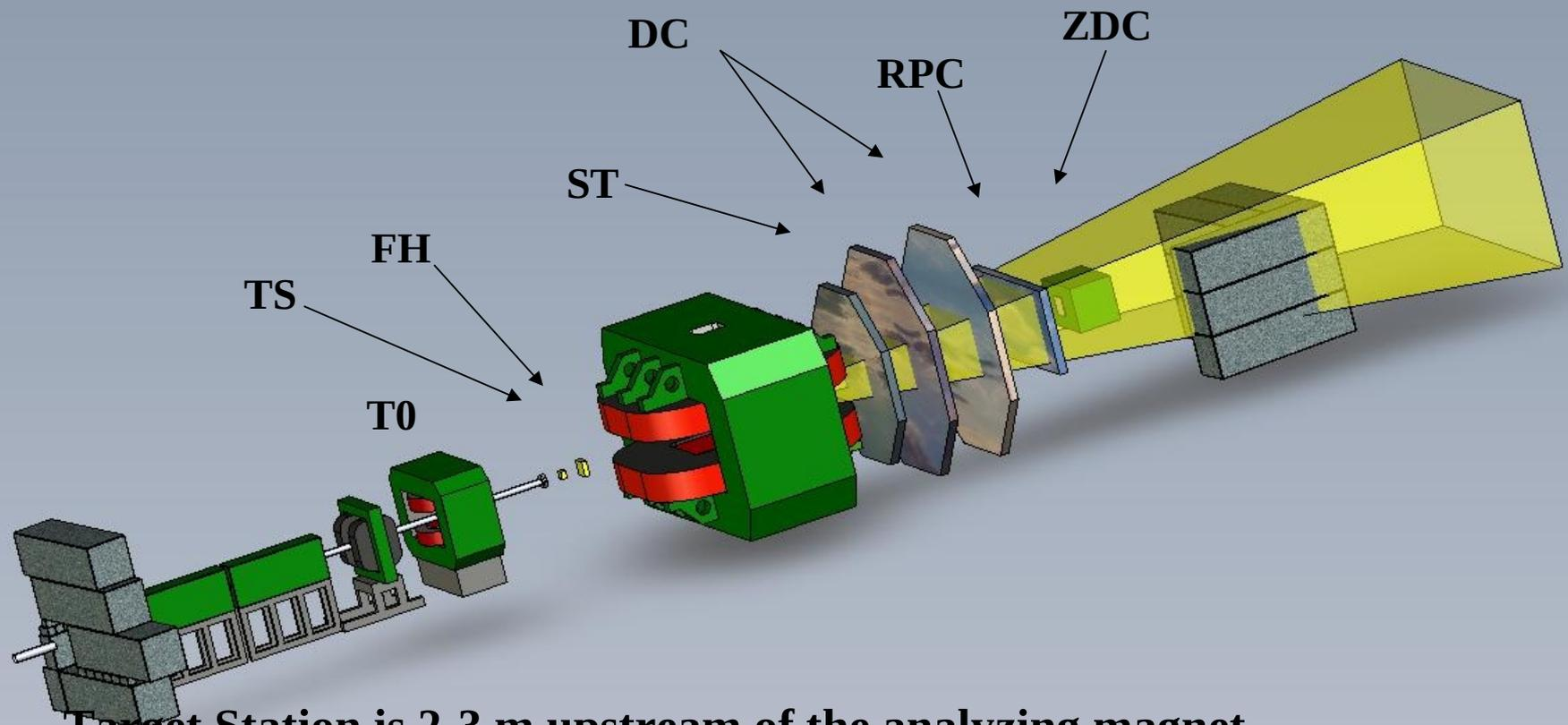
Target Station is 2-3 m upstream of the analyzing magnet
