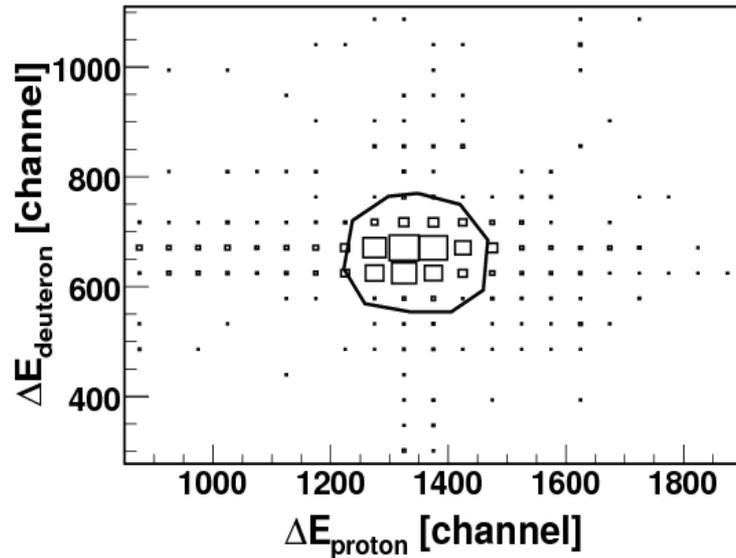
The correlation of the energy-loss signal for a pair of the deuteron and proton detector. The solid line is a graphical cut for the dp-elastic events selection.
