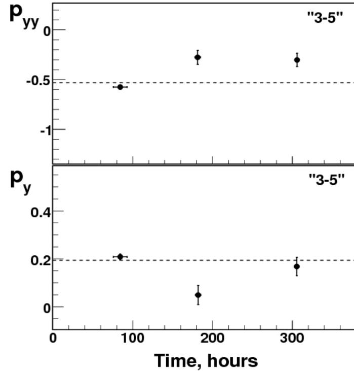
Tensor  $p_{yy}$  and vector  $p_y$  components of the deuteron beam polarization for "2-6" and "3-5" spin modes of PIS POLARIS as a function of the measuring time.
