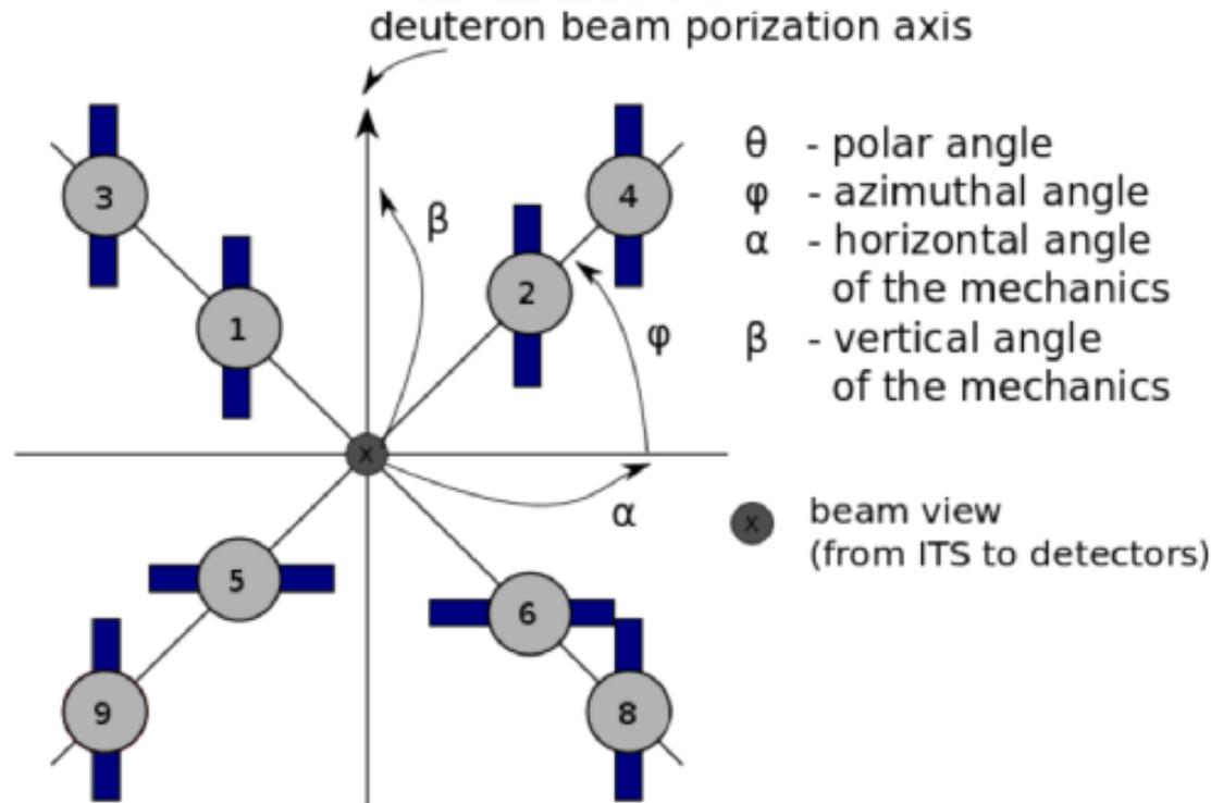
Detector placement is determined by polar  $\theta$  and azimuthal  $\varphi$  angles. Azimuthal angle  $\varphi$  have anticlockwise direction. Detector setup for the case of analyzing power investigation.
