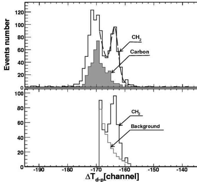
Selection of the dp elastic events by the time difference  $\Delta T_{\text{d-p}}$  between the signal appearance from deuteron and proton detectors with the criteria on the amplitude signal correlation.
