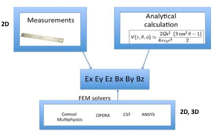
When calculating particle trajectories, an electromagnetic field can be specified analytically, in the form of a field map obtained as a result of measurements (2D maps) or as a result of model calculations (3D field maps).
