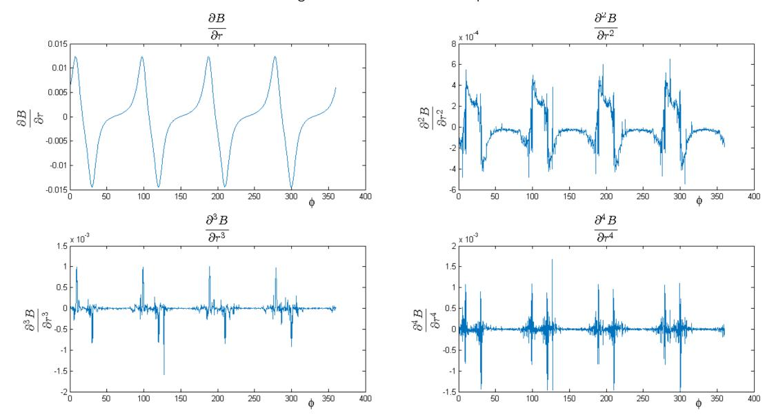
Derivatives of the magnetic field in the median plane taken with smoothing algorithms.
