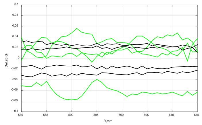
The four-sector structure of the magnet makes it possible to estimate the accuracy of the model calculation by comparing the magnetic field for identical parts of the magnet sectors (calculation in the 360-degree model).
