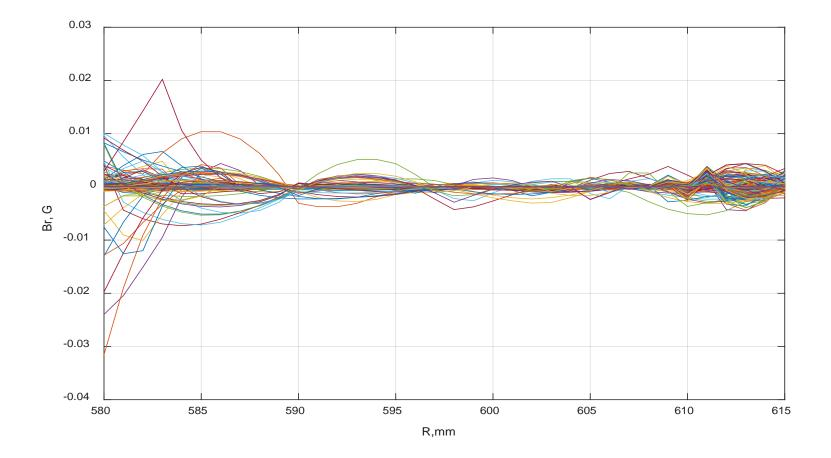
Theoretically, the components  $B\phi$  and Br are equal to zero in the median plane, the presence of components indicates an error value that is ±0.03 Gs in the extraction zone.
