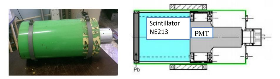
The **DEMON** neutron detectors use a **NE213** organic scintillator, which is coupled to a XP4512B photomultiplier tube. The effective diameter of the scintillator cell is 16 cm and the length is 20 cm. The effective diameter of the photo-cathode of the photomultiplier tube is 11 cm. A thick layer of aluminum tube (2 cm thick) is added between the cell and the outside housing of a 20 cm diameter steel tube in order to minimize the cross talk between detectors.
