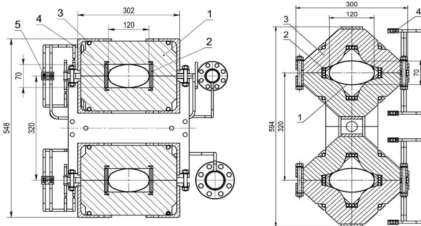
Cross-section of the collider magnets: Dipole magnet (left): 1 – lamination, 2 – SC coil, 3 – tube for cooling the yoke, 4 – beam pipe, 5 – bus bars; Quadrupole lens (right): 1 – beam pipe, 2 – half-yoke, 3 – lamination, 4 – bus bars. All dimensions in mm.
