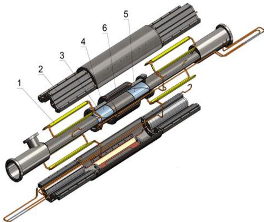
View of the doublet of the lenses. 1 – half-coil, 2 – half-yoke, 3 – beam pipe, 4, 5 – beam position monitors, corrector magnet
