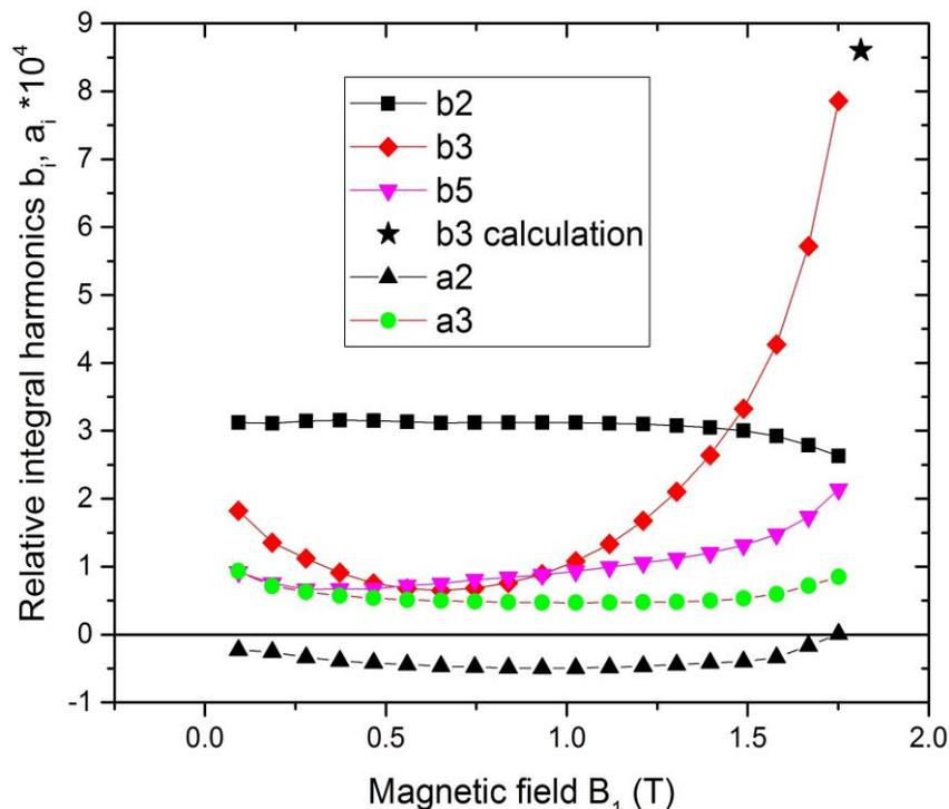
Relative integral harmonics of the magnetic field in the aperture of the NICA booster magnet at the radius of 30 mm as a function of the magnetic field in the magnet center.
