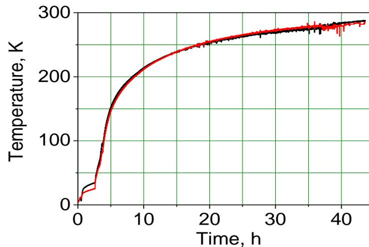
Cooling-down (left) and warm-up (right) of the dipole magnet for the NICA booster. Black line is inlet and red line – outlet of the magnet.
