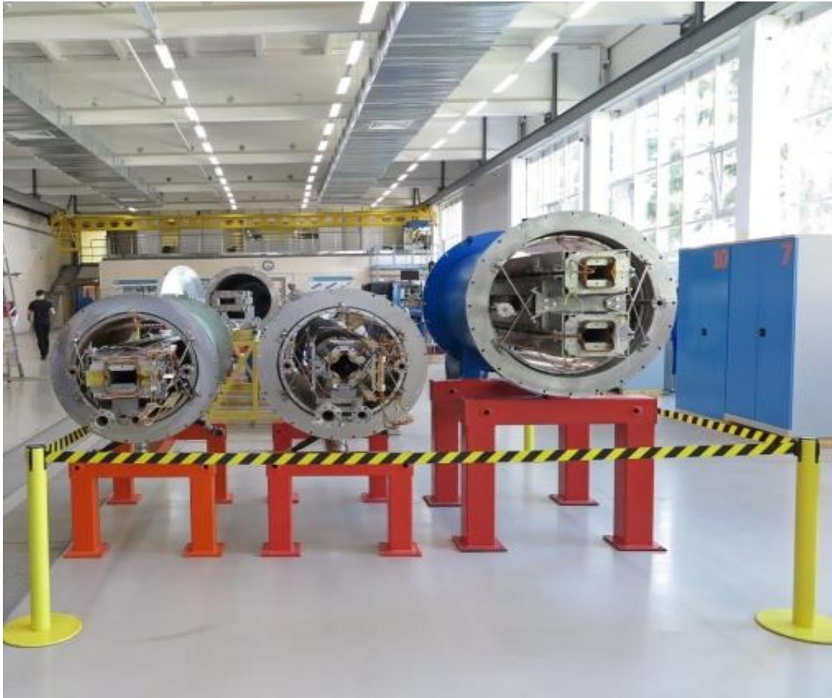
Series dipole magnet (left) and doublet (center) for NICA booster, and pre series dipole magnet for NICA collider (right).
