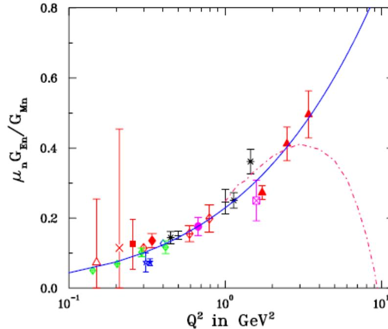
Approved experiments which will use the 12 GeV beam energy at Jlab in next future. The proton experiment uses recoil polarization as did the first 3 Jlab GEp experiments. The neutron experiments use a polarized  ${}^3\text{He}$  target (pink squares), and recoil polarization (pale blue circles).
