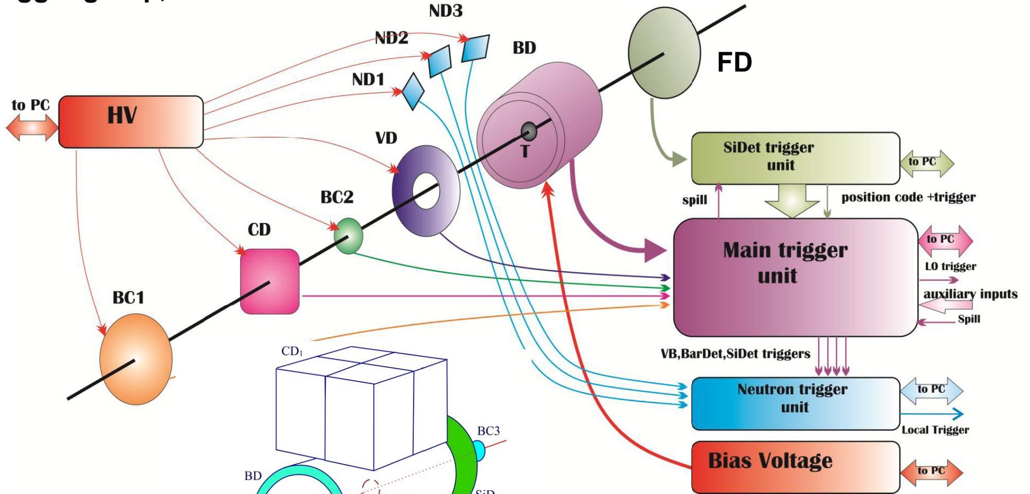
Trigger and T0 detectors for heavy ions
