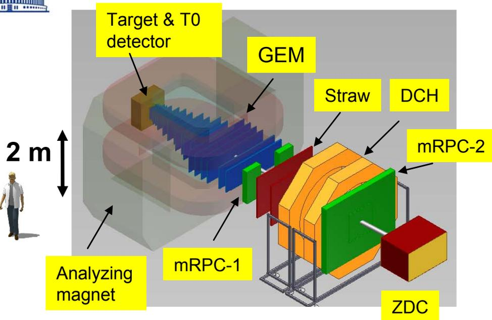
BM@N advantage: large aperture magnet (~1 m gap between poles)
