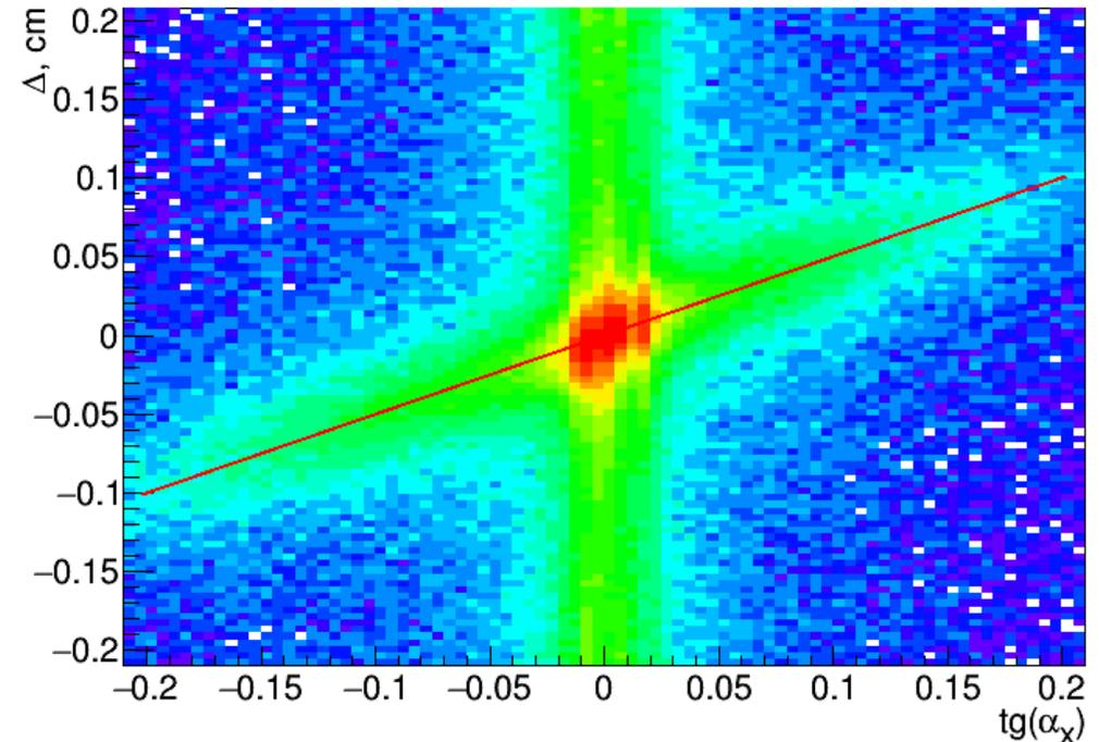
Residual distribution is inclined along X for shifted Z position.
