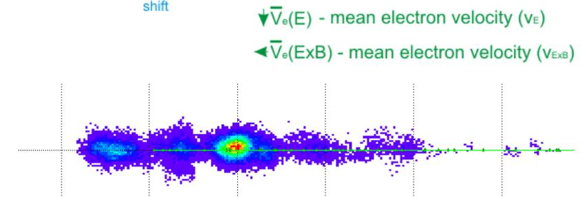
Profile of electron avalanche at the readout-plane (cluster).
